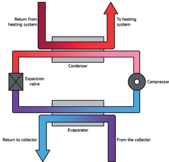
Fig. 9: Schematic process flow diagram for a ground source heat pump system
