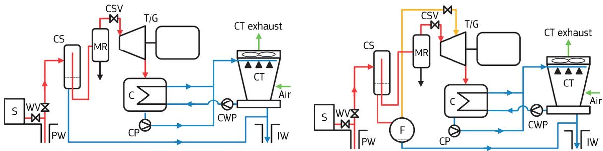
Fig. 5: Simplified flow diagram for a single flash (left) and a double flash (right) geothermal power plant. See text for details. Source: [DiPippo 2012], adapted
