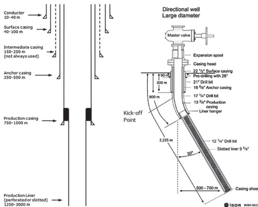
Fig. 7: Casing strings and liner in a typical geothermal well (left) modified from [Dumas et al. 2013]. The widths and depths are determined by geological and thermal conditions. A typical large diameter directional well from Hellisheiði, Iceland (right) [Sveinbjornsson & Thorhallsson 2014]
