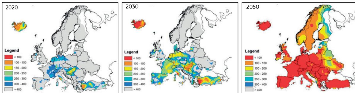
Fig. 2: Minimum levelised cost of electricity in 2020, 2030 and 2050. The economic potential for these scenarios translates to 21.2 TWh, 34 TWh and 2570 TWh within the EU. Source: [van Wees et al. 2013]
