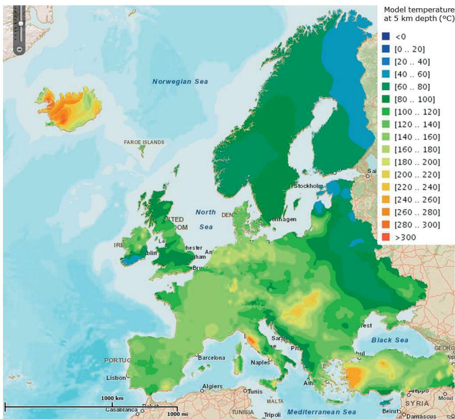
Fig. 1: Modelled temperature at 5 km depth in Europe (Source: Modified from GeoELEC Graphical Information System [ThermoGIS 2014])
