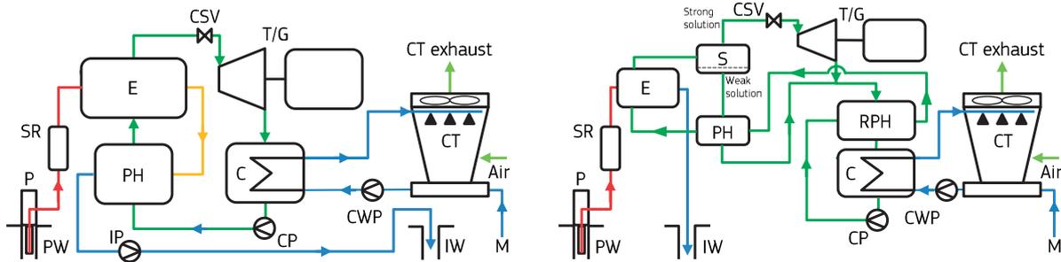
Fig. 6: Simplified flow diagram for an organic rankine cycle (left) and a kalina (right) binary geothermal power plant. See text for details. Source: [DiPippo 2012], adapted
