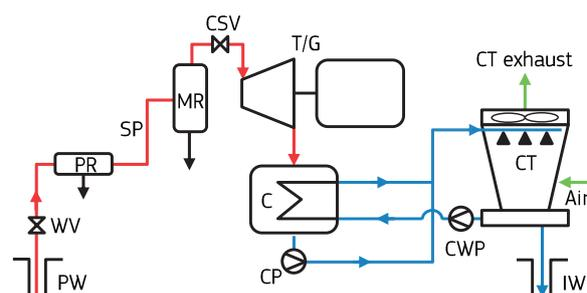
Fig. 4: Simplified flow diagram for direct steam geothermal power plant. See text for details. Source: [DiPippo 2012], adapted
