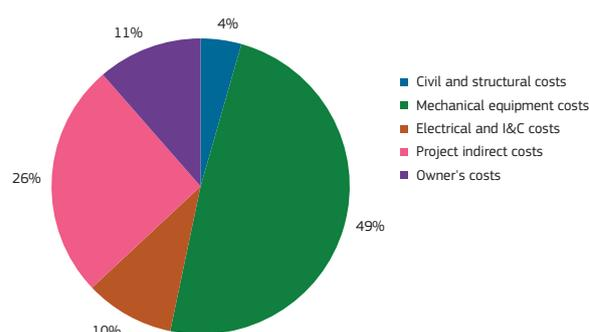
Fig. 37: CAPEX breakdown of an organic rankine cycle power plant
